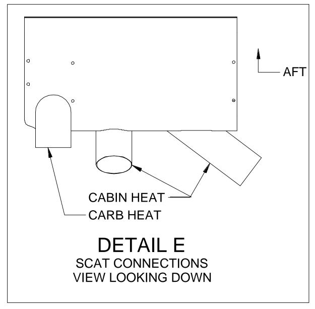
Combination shroud (50710) shown. When cabin heat is not installed or not regularly used, the Carb Heat Only Shroud (51711) must be installed. The Carb Heat Only shroud can be identified by the large cutout exposing the collector tubes and lack of cabin heat flanges.
