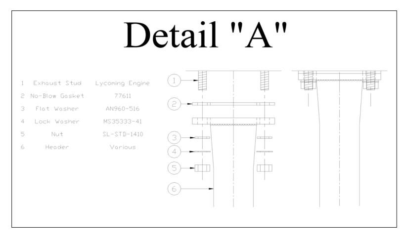
Note: Equivalent Stainless Steel Hardware may be substituted.
